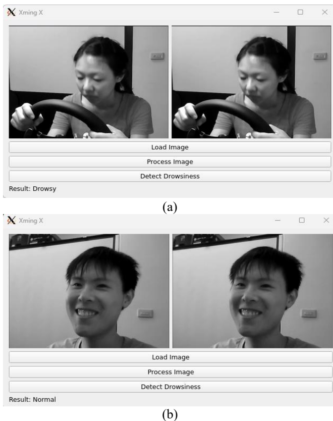
Figure 8. Drowsiness detection with ODT-DL GUI (a) Drowsy (b) Normal
