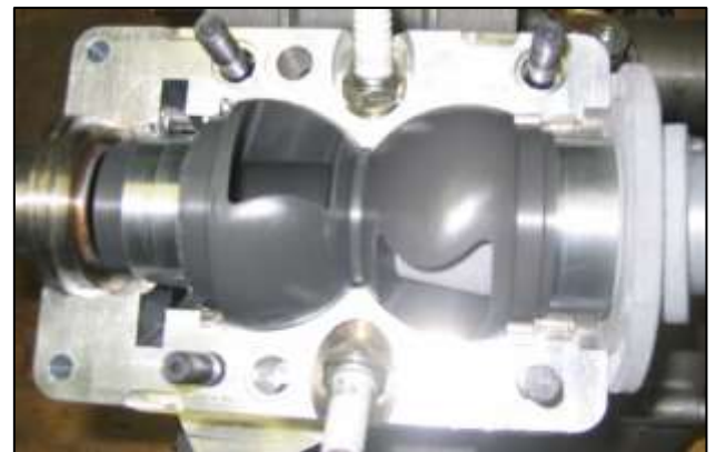
Figure 7. Actual manufactured Hofmann valve
