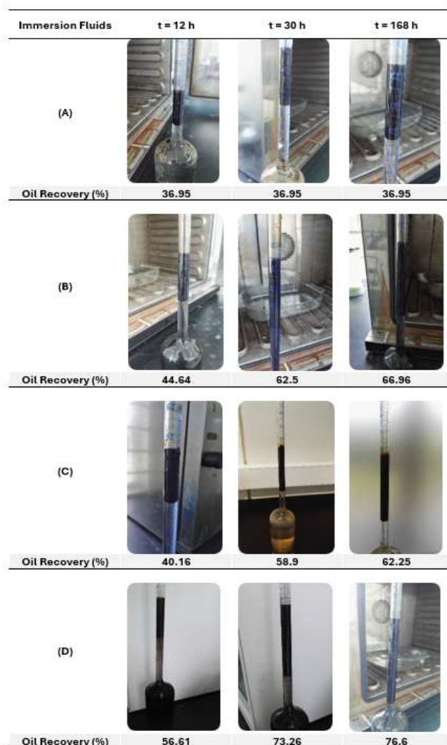
Figure 14. SI experiments at different stages of (A) Brine (30,000 ppm of NaCl), (B) GA-GNPs, (C) GA-SiO 2 , (D) GA-(SiO 2 -20% GNPs) nanofluids under HSHT
