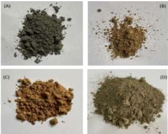
Figure 5. Plates 1A - D: Showing Burnt coal samples at different temperatures of (A) 900°C (B) 1000°C (C) 1100°C and (D) 1200°C
