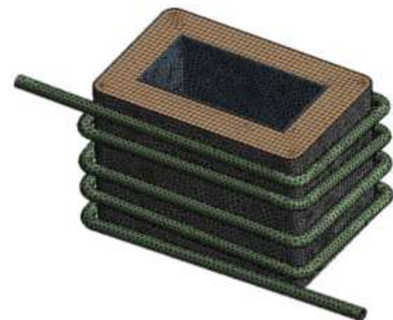
Figure 3. Battery geometry with meshing for CFD analysis
