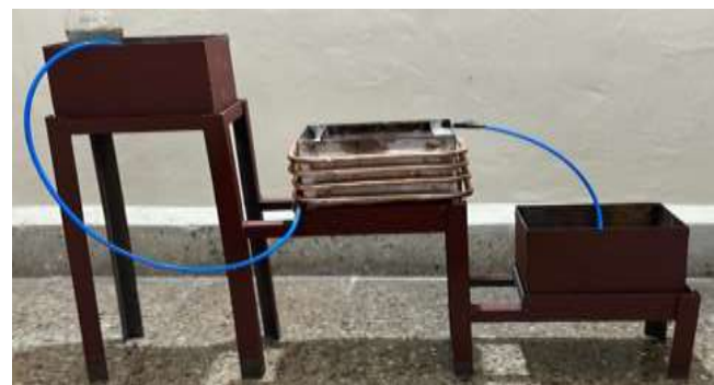
Figure 1. Experimental setup for battery cooling
