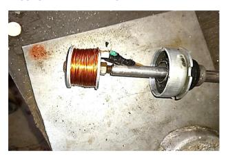
Figure 7. Vibrator (electrical motor with cam)
