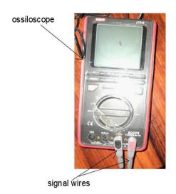
Figure 8. Portable oscilloscope
