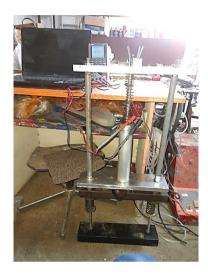
Figure 1. Semi-active suspension system
