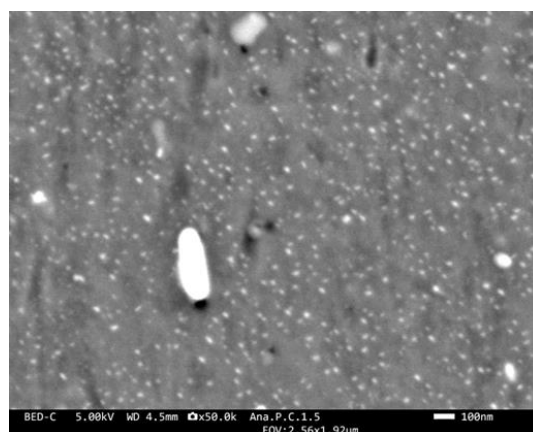
Figure 10. T6f temper-FEG-SEM observation. Fine precipitation
