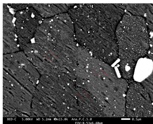
Figure 11. T6c temper-FEG-SEM observation. Precipitation bands framed by red dotted lines
