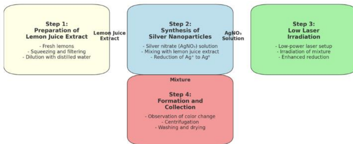
Figure 1. Schematic representation of the experimental process for the synthesis of silver nanoparticles using lemon juice extract and low laser irradiation
