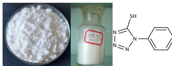
Figure 2. 1-Phenyl-5Mercapto-Tetrazole (PMT) inhibitor
