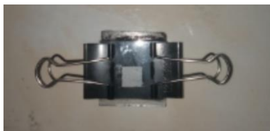
Figure 2. DSSC structure used for I-V measurement
