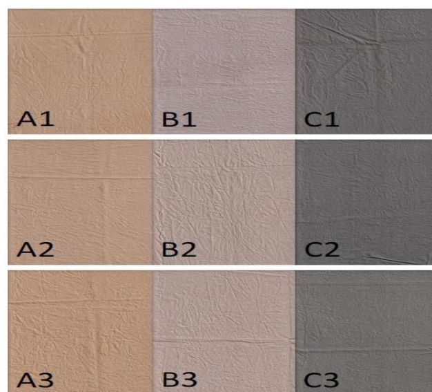
Figure 5. Color gradation of fabric resulting from dyeing and binding using senduduk fruit dye
