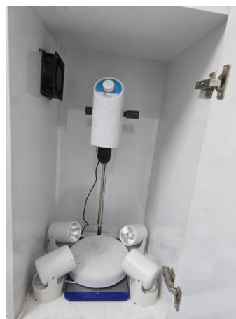
Figure 2. The batch reactor used in the photocatalytic degradation of MB dye
