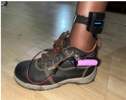
Figure 11. The piezoelectric energy harvesting footwear
