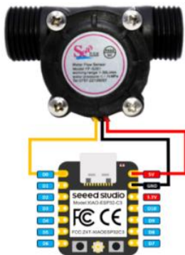
Figure 5. Schematic circuit for flow meter connection to the Xiao ESP32C3
