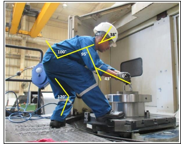
Figure 4. Measurement angle of REBA method for workpiece tightening activity
