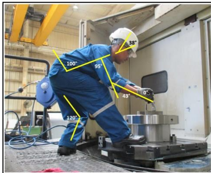
Figure 2. Calculation of limb angle in workpiece tightening activity
