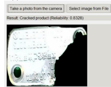
(b) Cracked product
