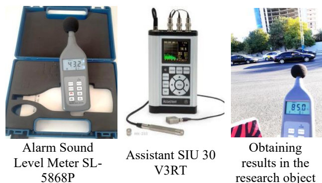
Figure 2. Measurement and comparative analysis of noise sources by contours on the streets of Samarkand and Tashkent City with noise measuring instruments
