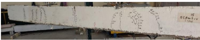
Figure 10. Crack pattern and failure mode of specimen BCR40VF1
