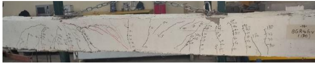
Figure 9. Crack pattern and failure mode of specimen BGR40VF1
