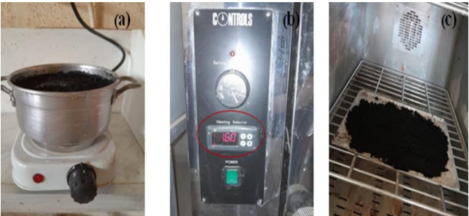
Figure 3. Schematic representation of the methodology employed for the aqua heat-treatment of rubber: (a) Rubber boiling; (b) Rubber drying
