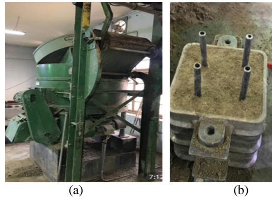
Figure 2. Sand casting equipment (a) Sieves and (b) Cast mold
