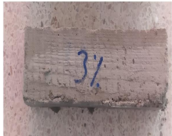
Figure 6. Prismatic samples of dimensions 4 × 4 × 16 cm for mechanical properties test
