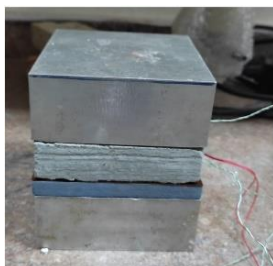
Figure 7. View and schema of asymmetrical hot plate device in steady state regime
