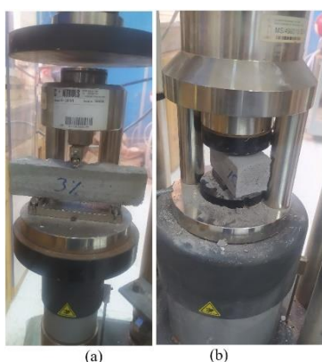
Figure 8. Device of mechanical tests: (a) tensile bending test (b) compression test
