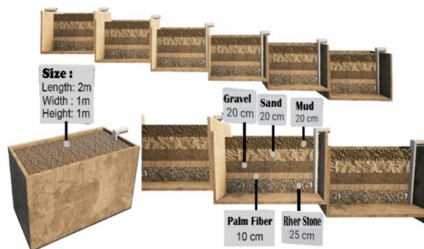
Figure 1. Design and construction of installation and materials used for wetland study
