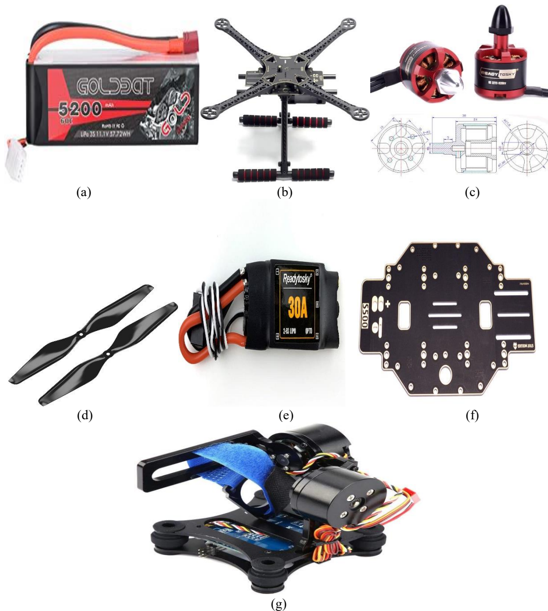
Figure 3. Selection of Some Key Components, (a) 5200 mAh LiPo battery, (b) Quadcopter frame, (c) Brushless motor, (d) Propeller, (e) Electronic speed controller, (f) Power distribution board, (g) Gimbal
