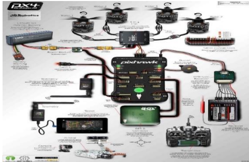
Figure 9. Interface of the Pixhawk flight controller to the other hardware components
