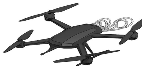
Figure 21. Vortex ring formation at high RPM
