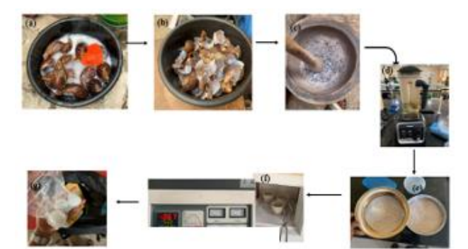
Figure 3. Cow horn preparation cycle (a) cleaning (b) drying (c) grinding (d) blending (e) sieving (f) carbonizing (g) packaging
