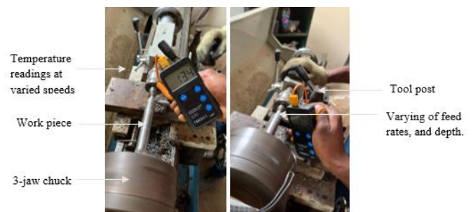
Figure 8. Machining to test viability of cutting tool
