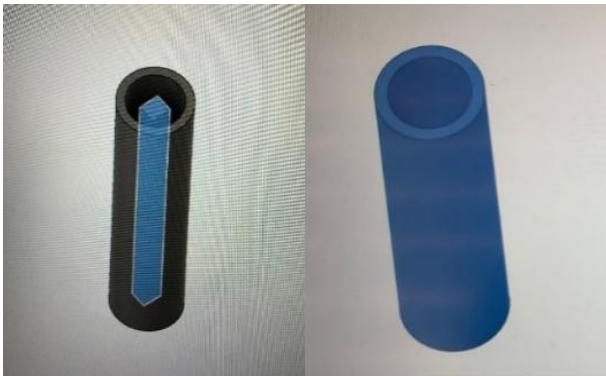
Figure 5. Calculation of fill volume (a) volume of tool (b) volume of steel housing
