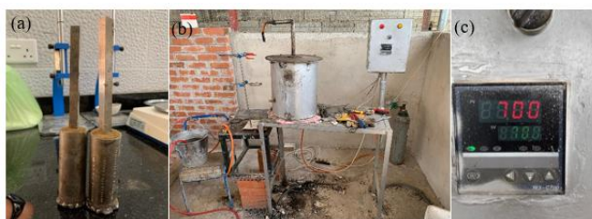
Figure 7. Case hardening of both samples (a) foundry clay for case sealing (b) heating reactor (c) heating at 700°C
