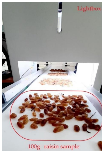
Figure 6. Outside view of the light box
