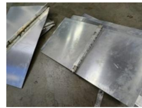
Figure 4. Specimens model for drop test
