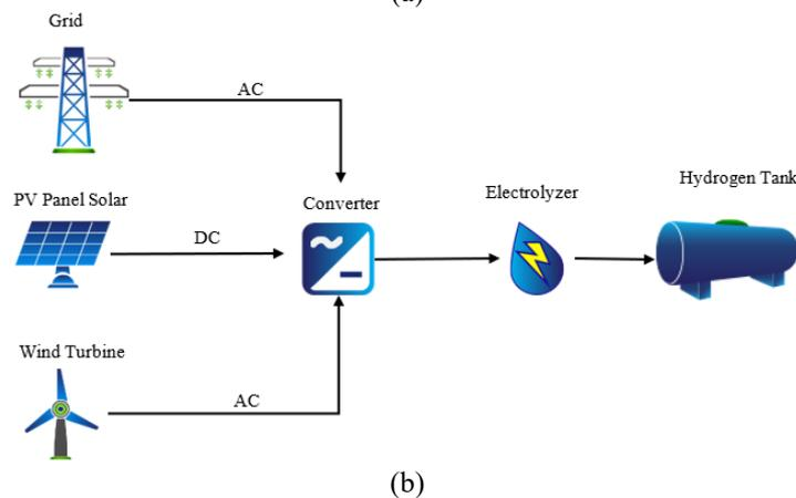
**Figure 1.** (a) Flowchart for HOMER Pro system, (b) System schematic [27, 28]
