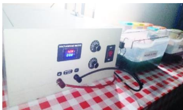
Figure 2. The electroplating process is carried out in the laboratory
