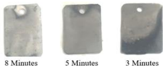
Figure 3. Macro photo of the substrate surface that has been electroplated with a current of 50 A
