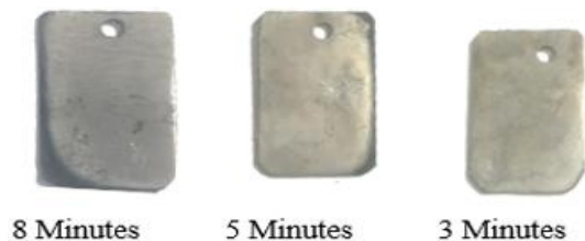
Figure 5. Macro photo of the substrate surface that has been electroplated with a current of 10 A
