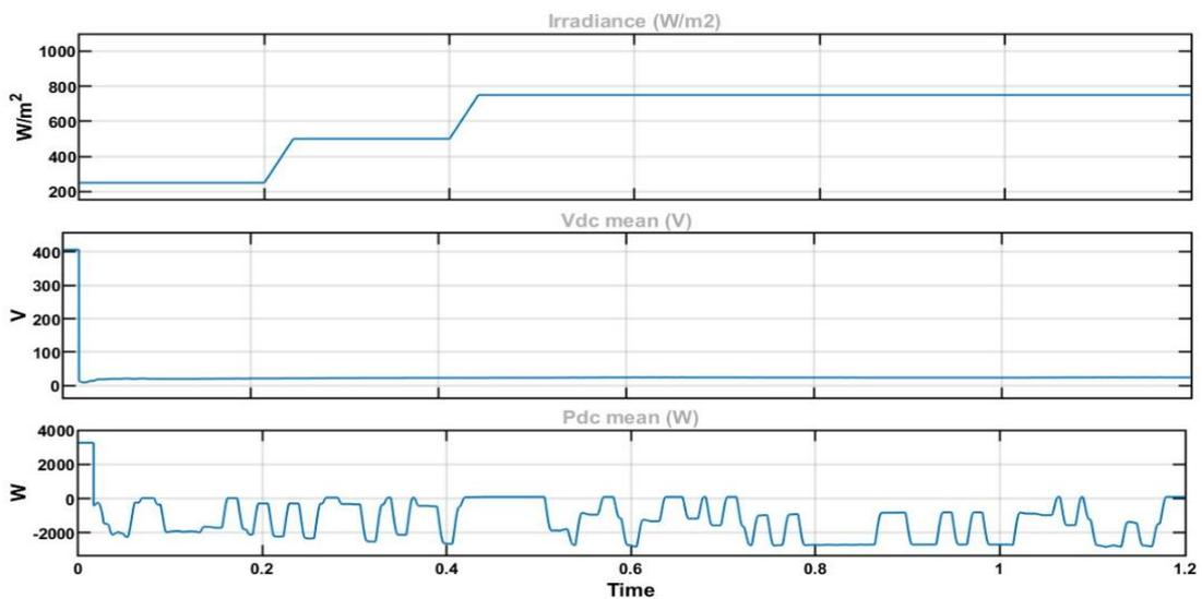
**Figure 7.** Voltage and power variations of a PV system under changing insolation conditions
