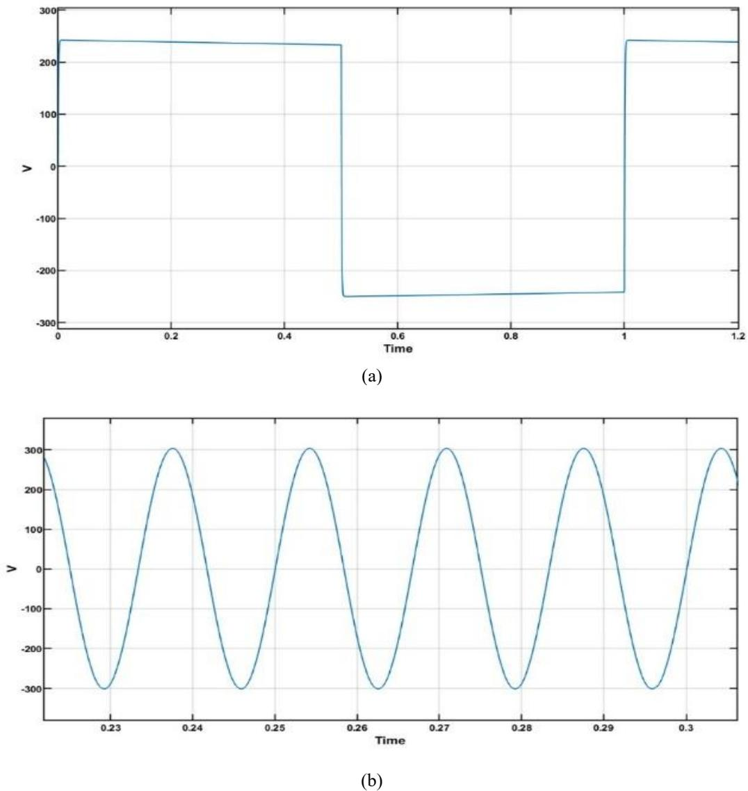
**Figure 10.** Graph wind turbine voltage of the inverter (a) before using (b) after using the LC filter
