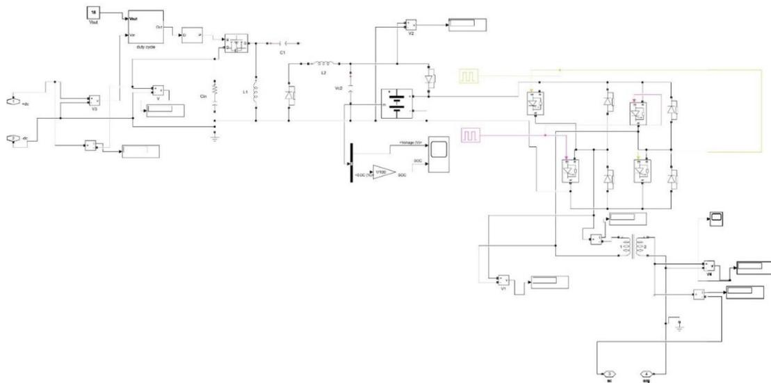
**Figure 5.** Simulink model of PWM inverter
