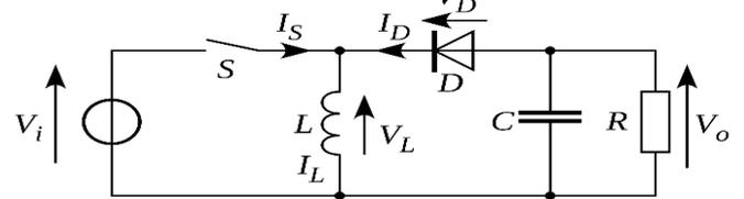
Figure 3. Ideal electronic circuit for a Buck-Boost converter
