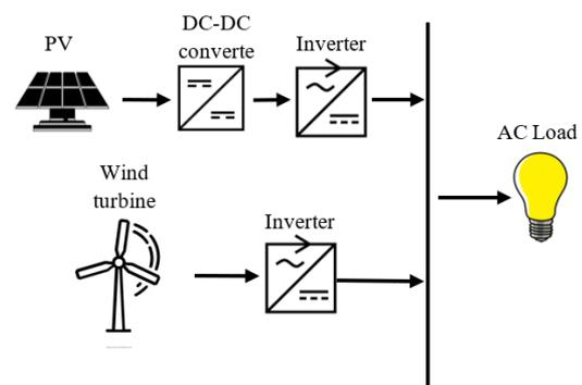
**Figure 1.** Simplified diagram of a stand-alone hybrid PV-Wind system
