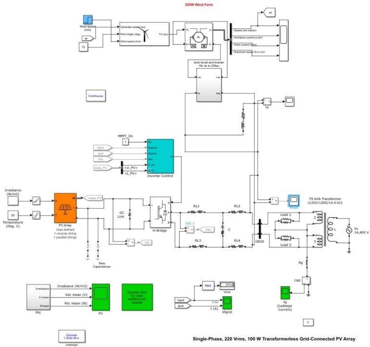
Figure 6. The modeling of a hybrid power generation system combining PV and wind energy
