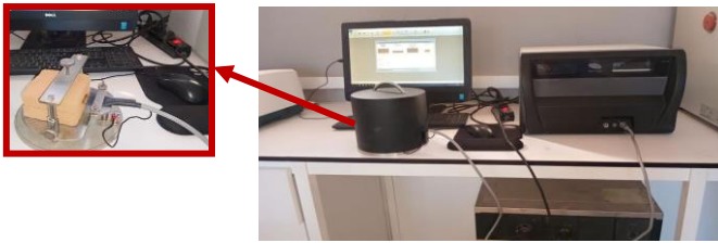
Figure 9. Thermal test on (10 \times 10 \times 2,5 \text{ cm}^3) prisms of adobe bricks
