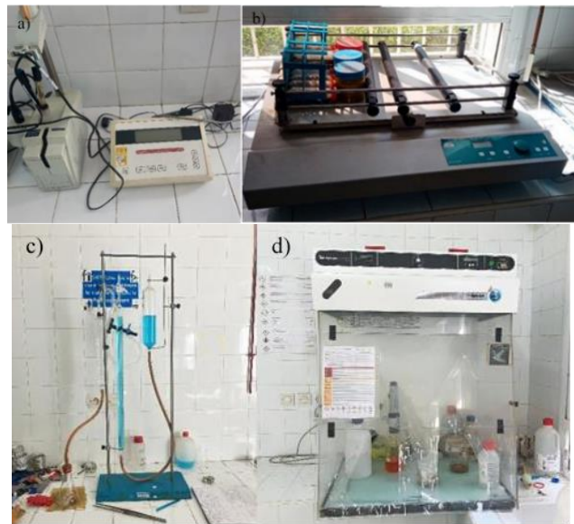
Figure 3. a. b) Materials used to measure pH, salinity, electrical conductivity, c) Calcium carbonate content, d) Organic matter
