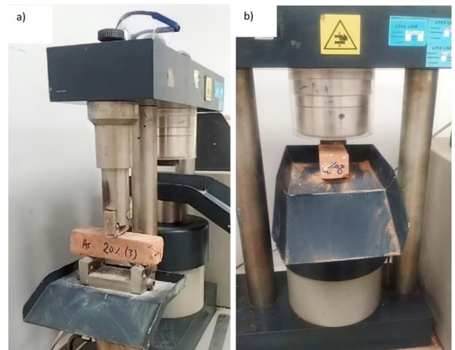
Figure 8. Mechanical test on (4×4×16 cm 3 ) prisms of adobe bricks
