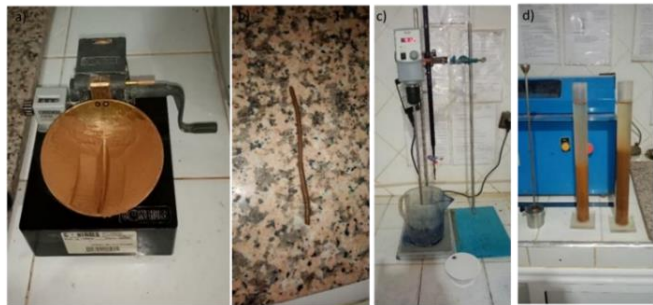
Figure 2. Techniques used to measure geotechnical soil properties: a. b) Atterberg limits, c) Methylene blue, d) Sand equivalent
