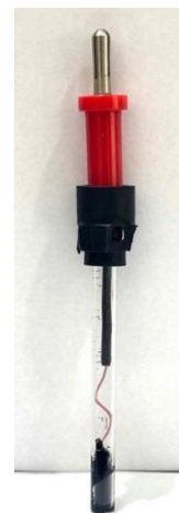
Figure 2. MgO-NPs carbon paste working electrode
