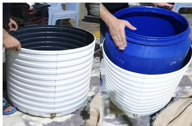
Figure 1. Prepare the large tank with one of the tanks to create the air gap
