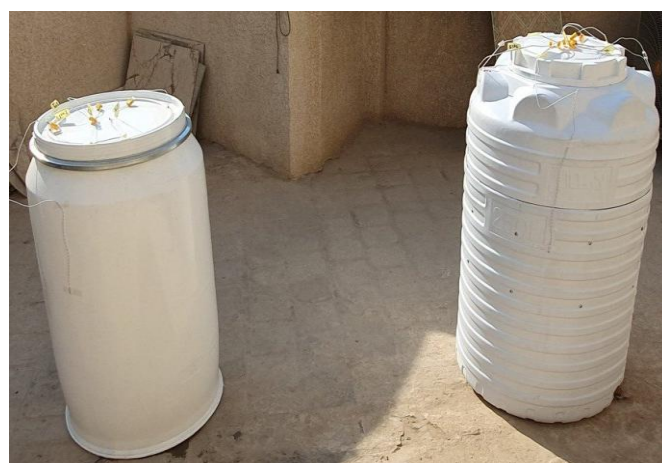
Figure 2. Experimental rig (the left tank without air gap and the right tank with air gap)
