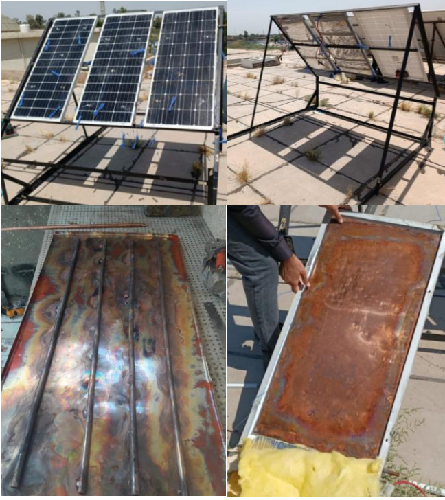
Figure 2. The utilized PVT in this experimental work with the applied copper collectors
