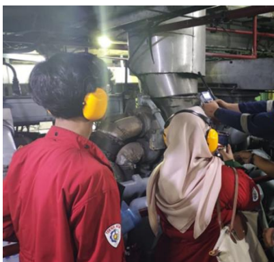
Figure 6. CO and CO 2 leak data collection using indoor air quality monitor probe
