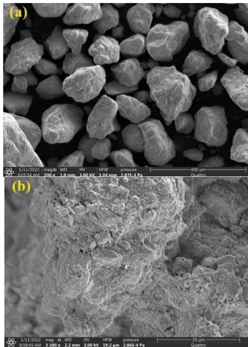
**Figure 3.** Scanning electron micrographs of materials: (a) Sand, (b) Kaolin
