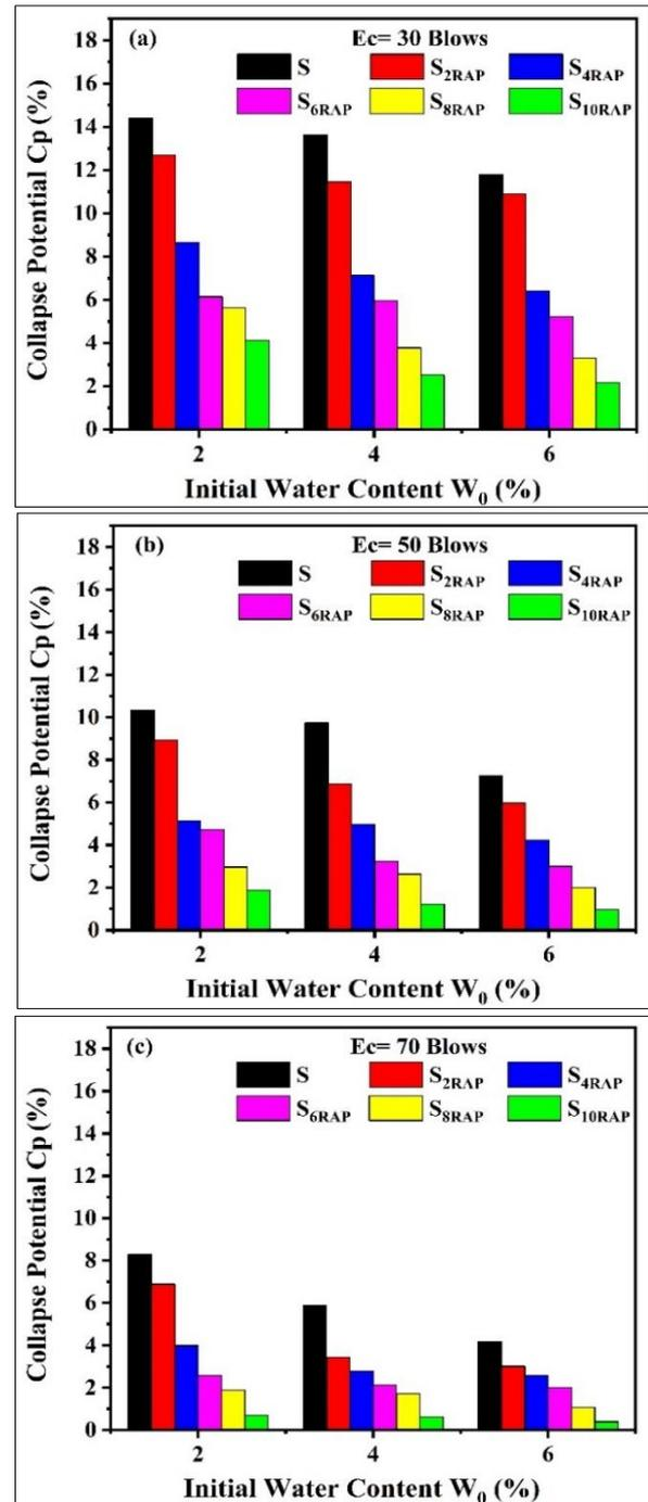
Figure 8. Effect of the addition of RAP on the collapse potential of soil at different  $E_c$  (a) 30 blows, (b) 50 blows, (c) 70 blows
