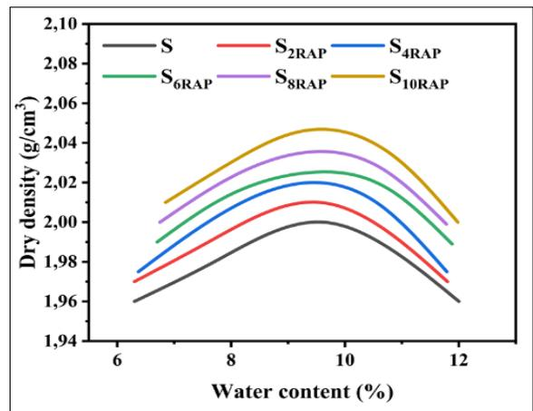
**Figure 10.** Effect of RAP on soil compaction
