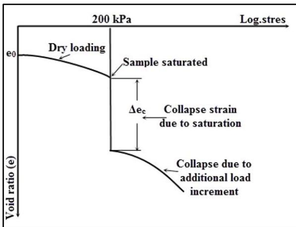
Figure 6. Simple oedometer curve
