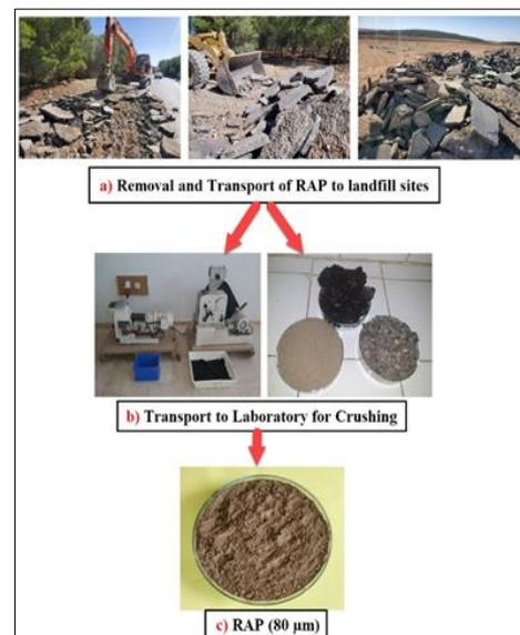
Figure 2. Schematic diagram of RAP preparation for experimental tests
