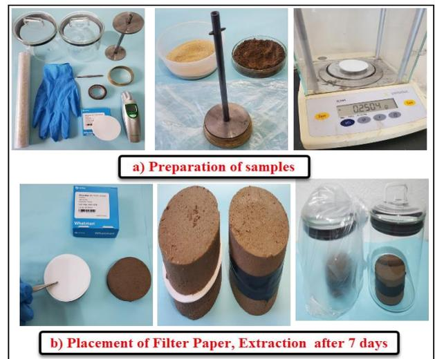
Figure 7. Suction measurement test by filter paper (Whatman ashless grade 42)
