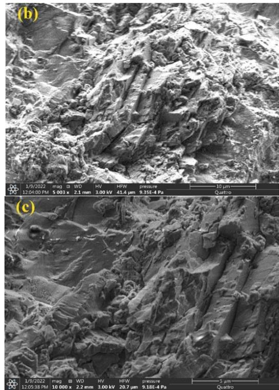
**Figure 11.** SEM pictures of treated soil with RAP (a) 3500x, (b) 5003x, (c) 10000x
