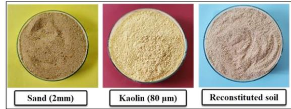
Figure 1. The main materials for preparing soil samples
