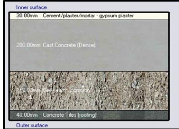
(b) Construction materials for roof (Ashti House)
