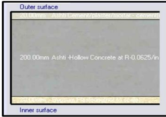
(a) Construction materials for wall (Ashti House)
