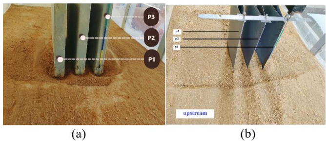
Figure 4. Experimental details when ( S/D_p=1 and \alpha=0^\circ ) for (a) rectangular piers and (b) lenticular piers
