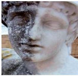
Figure 6. Greek marble head after laser cleaning without damage [36]
