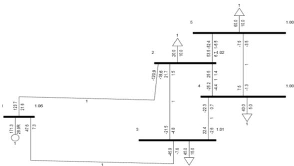
**Figure 2.** Initial load flow result of test bus system
