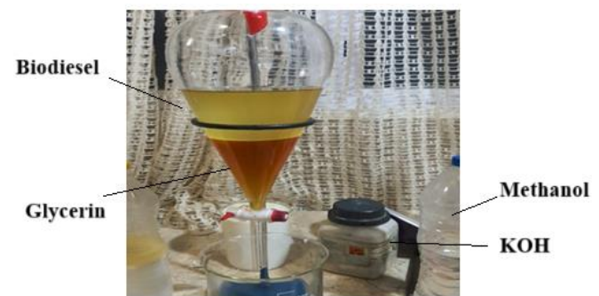
Figure 1. Separating biodiesel from glycerin after the transesterification process
