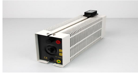
Figure 2. Simulated unbalanced supply using variable resistance control
