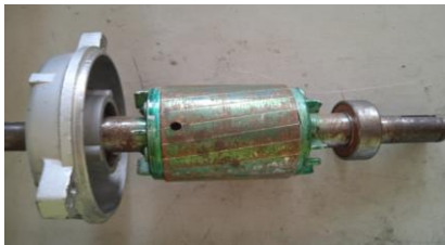
Figure 11. Experimental setup for internal unbalance (broken rotor bar fault)
