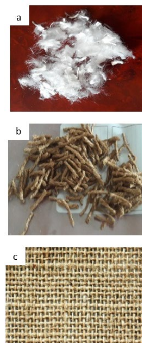
Figure 1. Different types of reinforcement: a) Polypropylene, b) Jute, and c) Woven jute fibers
