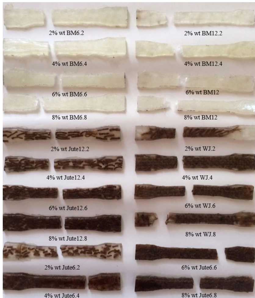
Figure 4. Tensile samples after the test
