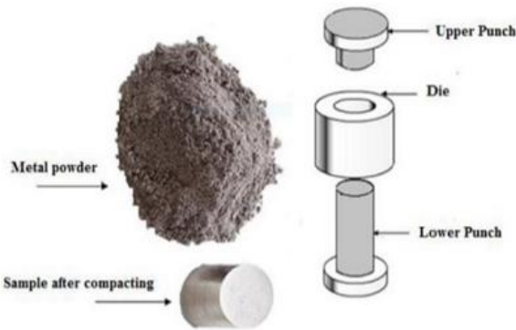
Figure 2. Sketch of single-action tool steel mold [24]
