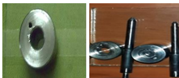
Figure 9. Molds utilized to generate special hardness analysis sample preparations
