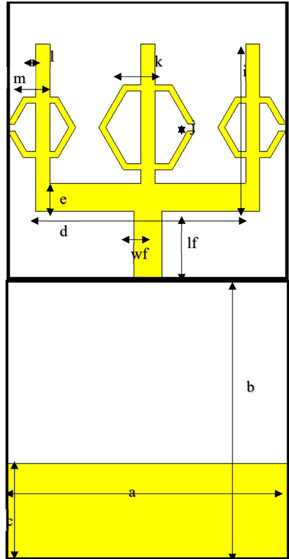
Figure 3: SRR-inspired antenna array parameters
