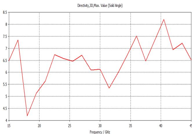
Figure 12 SRR-inspired antenna array directivity vs. frequency
