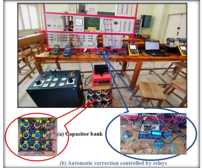
Figure 13. Implementation design for investigating parallel compensation with smart automatic Arduino unit
