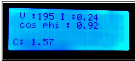
Figure 14. Electrical characteristics of an ohmic-inductive load after correction
