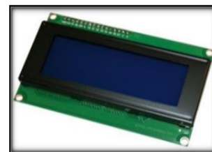
Figure 6. 20x4 LCD display
