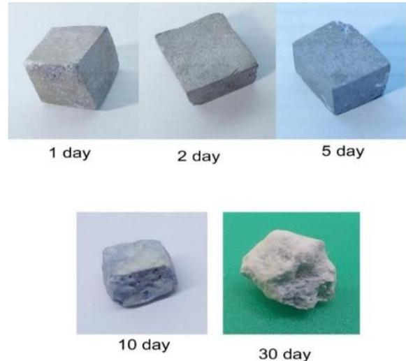
Figure 9. AZ91 alloy sample after different immersion time
