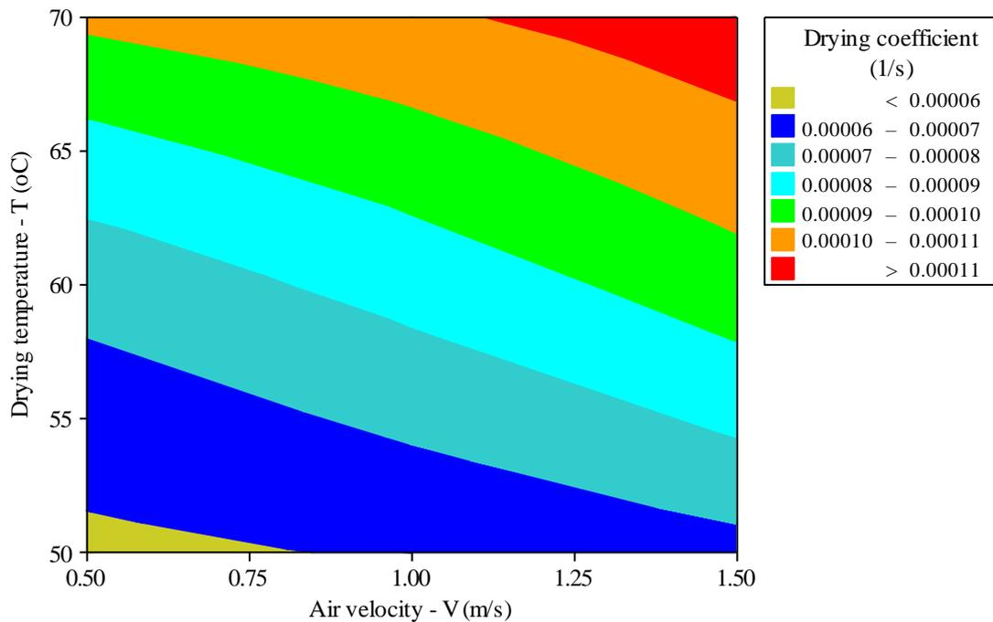
**Figure 2.** The variation of drying coefficient with air velocity and drying temperature
