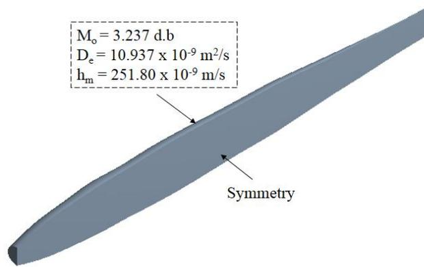
Figure 4. The computed domain and boundary conditions
