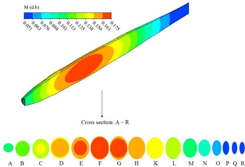
Figure 6. Moisture content distribution inside fish
