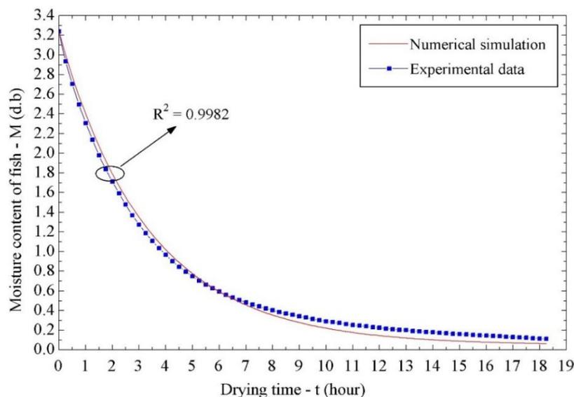
**Figure 7.** The variation of moisture content with drying time according to experiment and simulation
