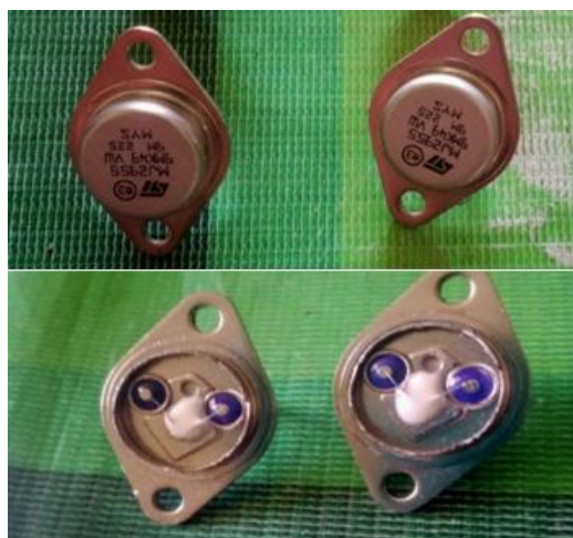
Figure 2. MJ2955 transistor construction
