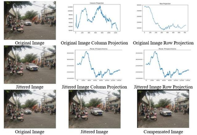
Figure 8. EIS grayscale projection preprocessing and stabilization output
